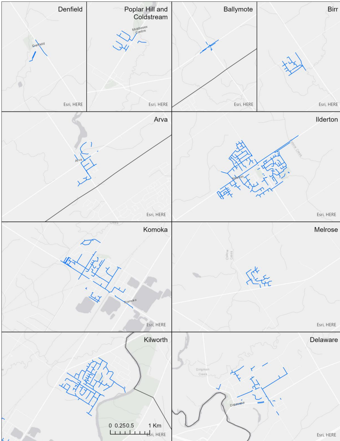
Figure 2-12 Stormwater Mains - Communities
