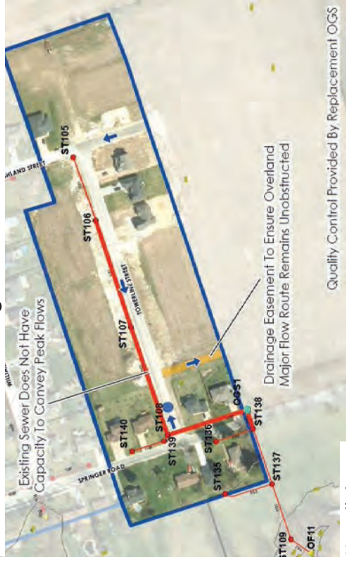
Alternative 2 – Abandon Municipal Drain & Negotiate Drainage Easement*
