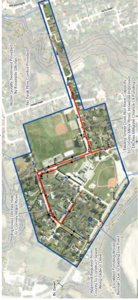
Alternative 3A – Improve Roadside Ditches, Provide 100-Year Storm Outlet, and Abandon Municipal Drain*
