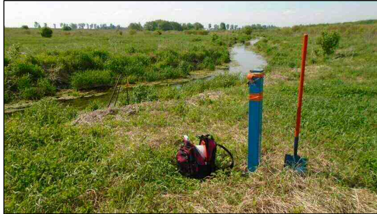
Photo 1. Looking downstream at Medway Creek on May 22, 2022, monitoring well MW2 is in front and staff gauge SG2 is to the left of MW2.
